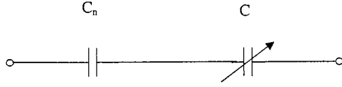
Fig. 2. Series association of a negative capacitance C_n and a tunable positive capacitance C .
